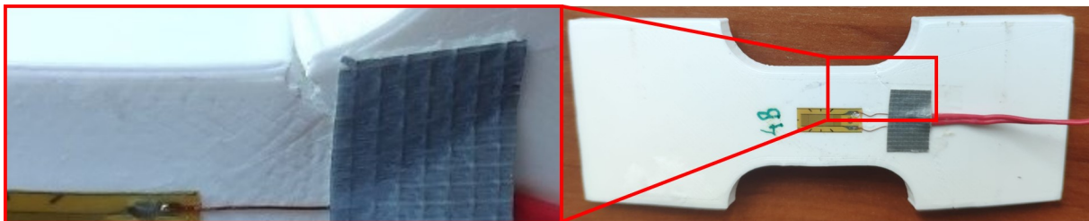
Figure 6.5: Crack at the root of the transition of specimen 1B
