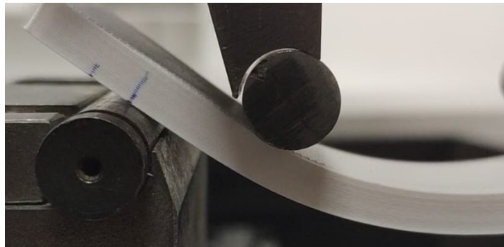
Figure 6.3: Gap between the loading roller and the test fixture at high values of deflection
